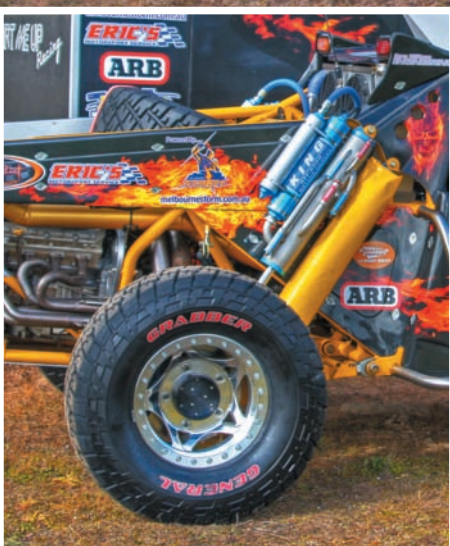
(Left) A combination of King Bypass and coilovers manage the Porters suspension travel. (Above) A pair of Motec ECU's run the BMW V10, feeding to info direct to the digital dash mounted amidst a sea of carbon fibre.
