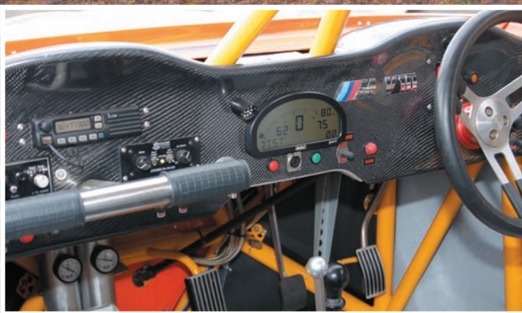
(Left) A combination of King Bypass and coilovers manage the Porters suspension travel. (Above) A pair of Motec ECU's run the BMW V10, feeding to info direct to the digital dash mounted amidst a sea of carbon fibre.
